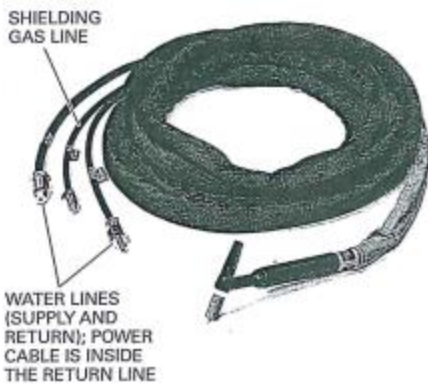
WATER-COOLED GTAW TORCH
