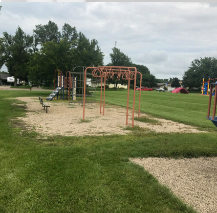
Dangerous short distance of play equipment from edge of safety surface
