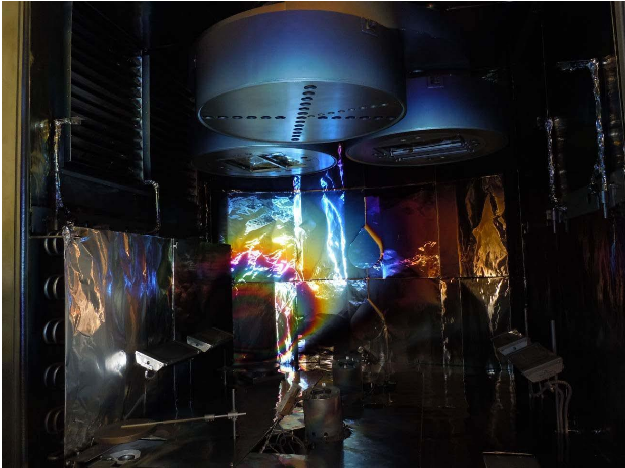
Figure 1 – JJMO Mirrors in Goodrich Coating Chamber Prior to Coating
