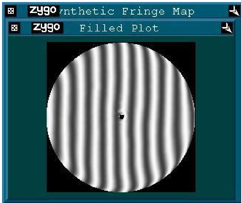
Figure 5 – Example Interferometry Data for JJMO 8 inch Mirror – Deviation from Ideal Surface
