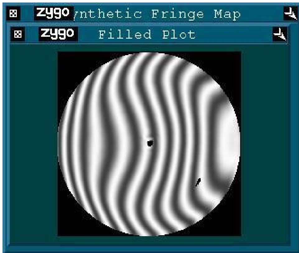
Figure 4 – Example Interferometry Data for JJMO 8 inch Mirror – Deviation from Sphere
