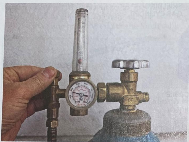
Figure 32 Adjusting the flowmeter.
